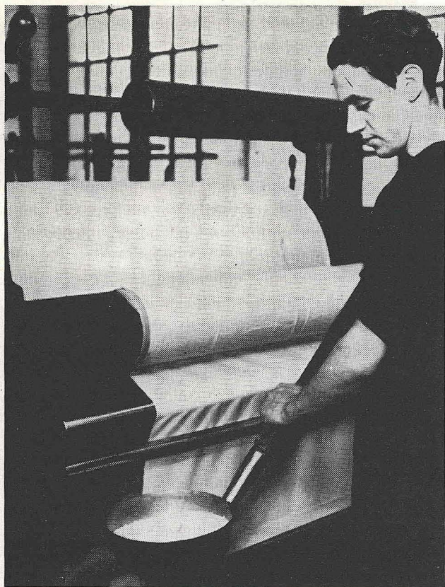
Figure 7. Scouring with Sodium Metasilicate Solution on Jig
